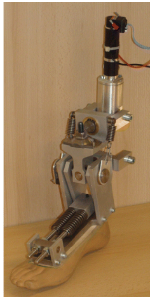
Figure 17. Ankle Prosthesis prototype developed by UCL-Belgium [1]
